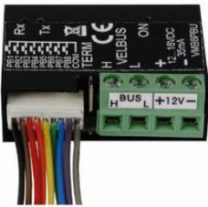
The universal VMB8PBU input module can easily be mounted behind push button panels of your choice. This module allows you to connect up to eight switches, each with feedback indicators (if LEDs are fitted, sold separately). Feedback can also be configured with a night mode. Please note that the wires connecting the push buttons should not be extended.
